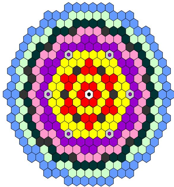
**[Reactor core loading pattern]**
